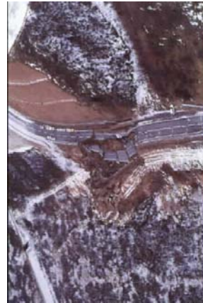
a part of road embankment constructed curved slope was slid away, in 1993 Kushiro-oki Earthquake.
